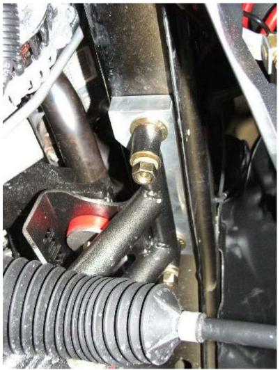
Once we were done with 1 side we moved to the other and did the same exact thing making sure that the engine and transmission were still supported with the transmission jack supports.
