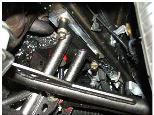
Now for the rear K-member spacer we made sure there was enough space to slide the spacer in. Using the supplied 2.5" bolts we bolted them through the rear mount of the K-member and spacer to the frame.
