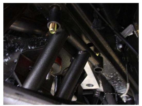
Then we used the long bolt and washer supplied with the kit and dropped it through the frame, spacer and K-member from the top. Using the supplied washer, locking washer and nut we then tightened up the nut on the bolt. Do not fully tighten the nut until you've finished placing the spacers on the front and rear K-member mounts as tightening them before installing the rear K-member spacers will not give you the ability to adjust the K-member if needed.
