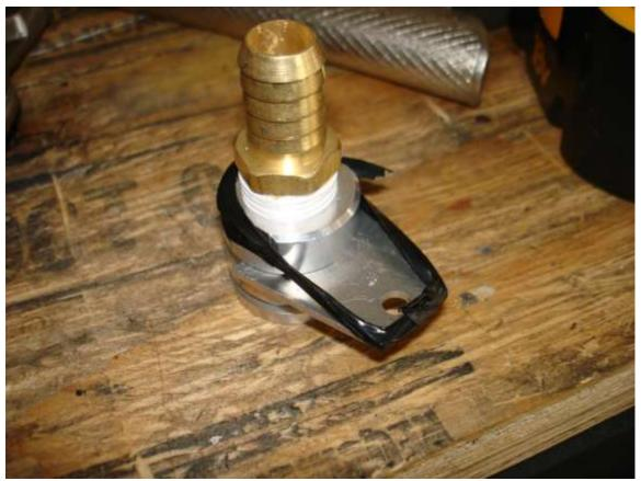
. A snug tightening will suffice. Do not over tighten. Place the supplied O-Ring on the bottom groove of the aluminum fitting and lubricate with petroleum jelly. Place the supplied blue silicone hose over the barbed fitting and secure with a hose clamp. This is how the assembly should be installed in the cylinder head. Make a note of how the hose clamp will be located once in place in order to have adequate access to tighten the clamp.
