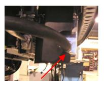
31) Re-attach the factory hose to the lower heat exchanger outlet, and attach the pump inlet hose, trim to fit if needed, to the pump.
