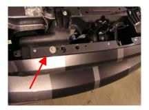
10) Lift the top of the bumper up and over the tabs. Then, slide the whole bumper cover forward and off of the vehicle. 11) Grab the foam bumper core and pull straight out to free the 4 plastic clips. Be careful not to damage the clips or the foam core.
