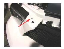
11) Grab the foam bumper core and pull straight out to free the 4 plastic clips. Be careful not to damage the clips or the foam core.
