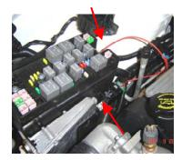
35) Mount the in-line fuse to the strut tower using the preexisting bolt. The cover should be reinstalled onto the fuse panel
