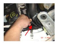
36) The ground cables should be connected to the bolt on the radiator support, which is shown below. The weatherpack connectors can be connected to the fans at this point.
