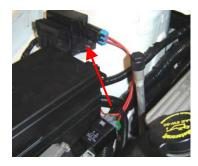
36) Run the wiring harness along the engine side of the fuse box up to the passenger side of the radiator. The harness will then go through the radiator support by the horns.
