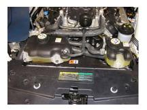
2) Remove the coolant tank cap from the heat exchanger coolant tank.
