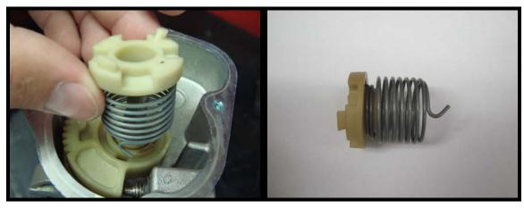
16. Install spring and plastic adapter to throttle body. \*\*Note that the tail of the spring locates into the hole in the brass gear.
