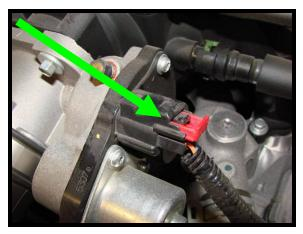
Throttle Position Sensor. Connect TPS connector to TPS sensor, lock red latch in place.
