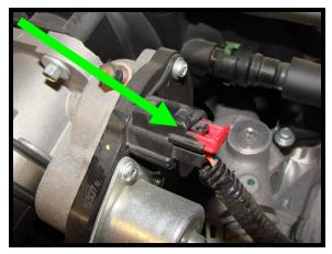
Throttle Position Sensor. Carefully pull red tab out, squeeze the connector and then pull the connector away from connection.
