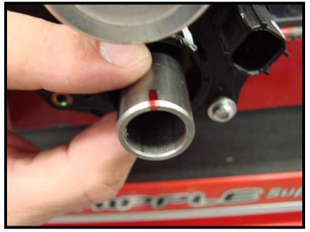
20. Rotate tool approx. 220 degrees. While close to the 220deg rotation, slightly pull the tool away from electric cover, this will let plastic adapter lock into place. If you inspect the plastic adapter, you'll notice there are 2 tabs that lock it in place. One small, one large, verify that this is correct before proceeding.
