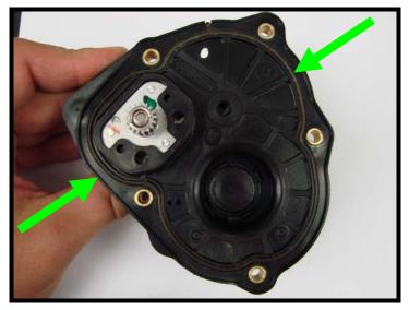
Install electric motor cover to new mono blade throttle body. Utilize the (5) factory torx bolts to secure in place.
