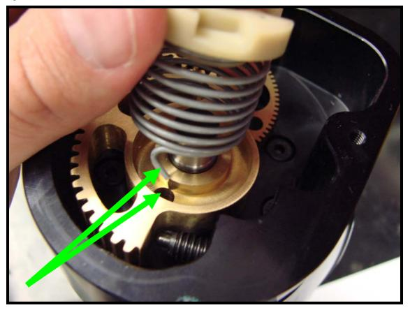
17. If oring fell from throttle body electric motor cover, reinstall using a very light amount of grease.
