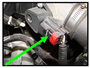
24. Install air inlet tube, secure (2) hose clamps.
