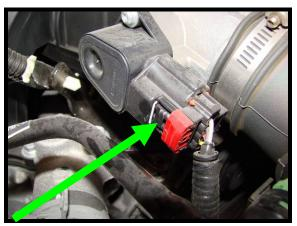
5. Disconnect plastic breather hose from air inlet tube. To release, push green tab on bottom side and then pull.
