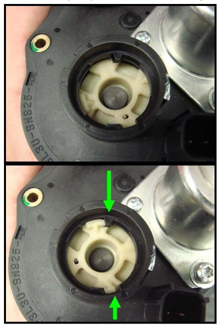
21. Reinstall the plastic inspection cover by carefully snapping into place.
