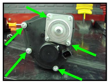
19. Install the spring rotation tool, into inspection hole. Using a marking pen, mark the top of the tool so you have a reference when rotating part.
