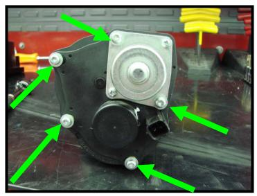
14. Using a small flat head screw driver, carefully remove the inspection cover from electric motor cover.
