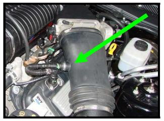
6. Loosen factory hose clamps (2) that secures air inlet tube to stock throttle body and mass air flow sensor.
