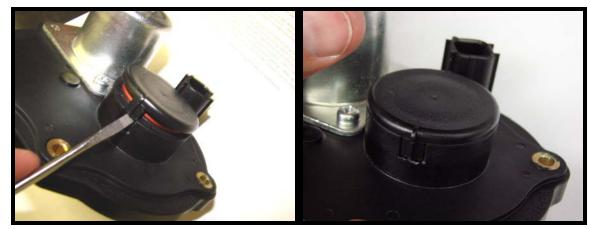
15. Remove the throttle spring and plastic adapter from throttle body. If this comes apart while removing cover from stock throttle body, then see picture below. The small end of the spring goes onto the plastic adapter. The spring locks into the plastic adapter with the tail of the spring locating into plastic adapter hole.
