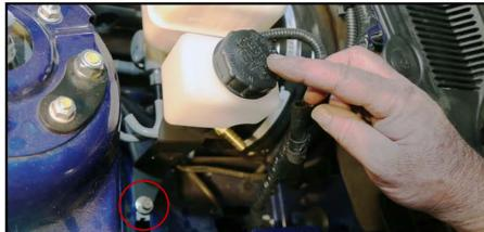
**Step 5:** Install hose on to new reservoir fitting. First slide tube in to place, then reinstall clamp in stock location.
