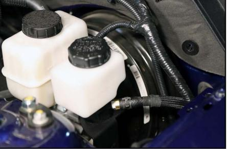
**Step 6:** Once installation is complete, fill new reservoir with DOT 3 brake fluid. Finally, pump clutch two or three times to ensure proper disengagement.
