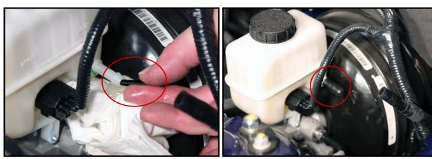
**Step 3:** Remove the lower nut from master cylinder with 13mm socket. Next install the clip nut into the existing hole behind shock tower.
