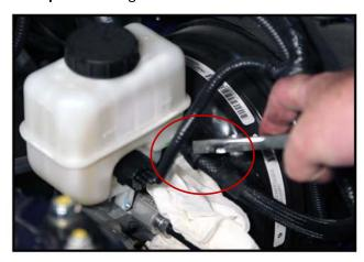
**Step 2:** Install the rubber cone seal. Once in place, install the rubber cover boot to ensure seal.
