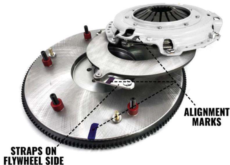
Install the floater onto the studs. Be sure to note the alignment marks. ***Floater straps must be on flywheel side.*** Install the three nuts and tighten to 25 ft. lbs. Check the disc clearance at this time. Insert the pilot tool and rotate the disc. There
