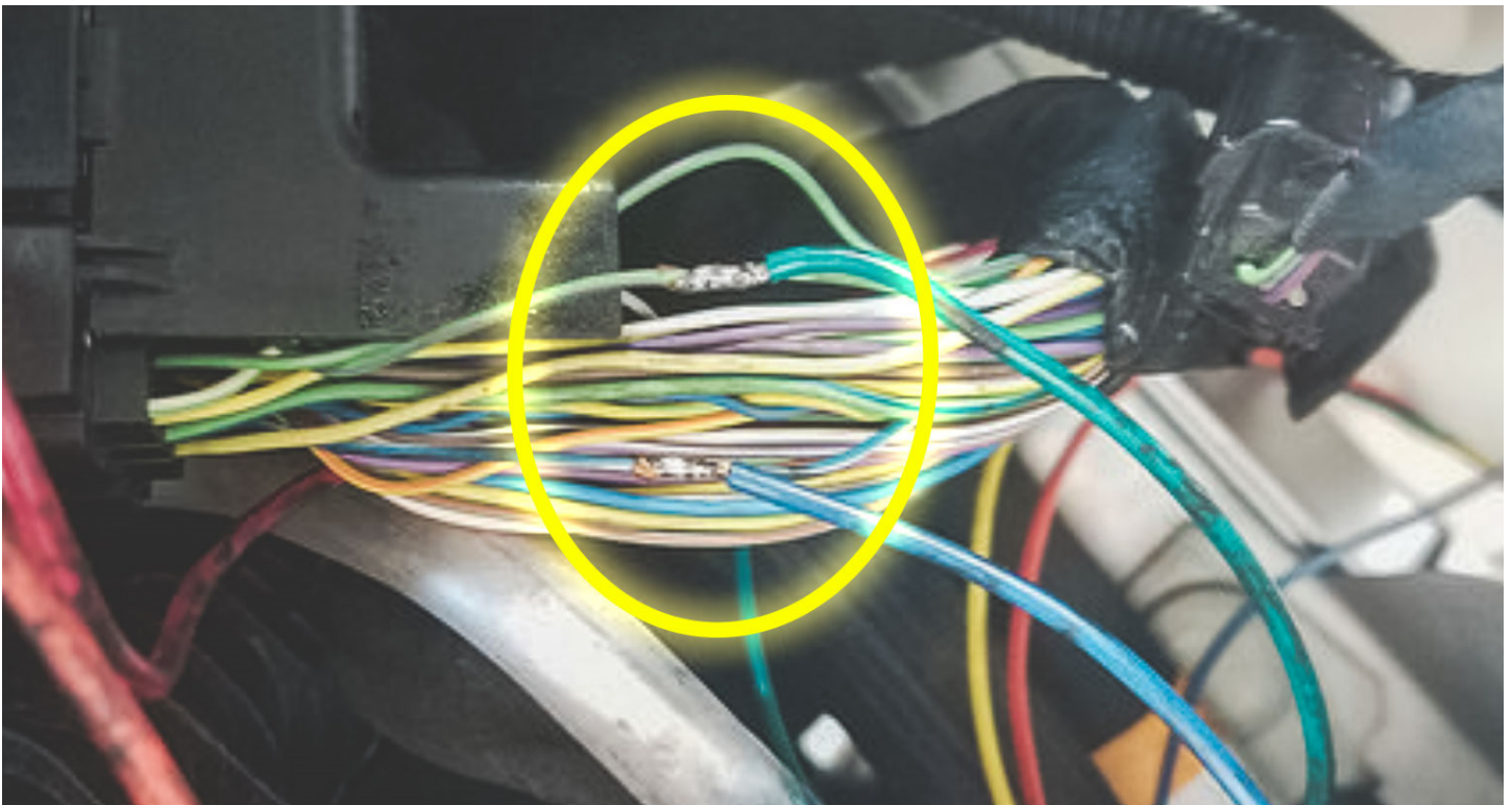
WOT Box BLUE and GREEN wires connected.
