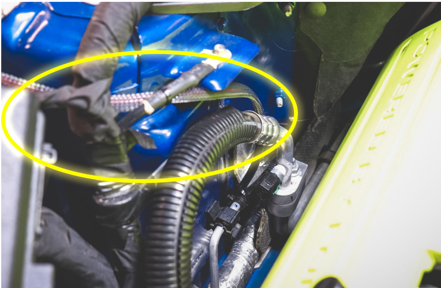
Route wires up into engine bay along passenger side.
