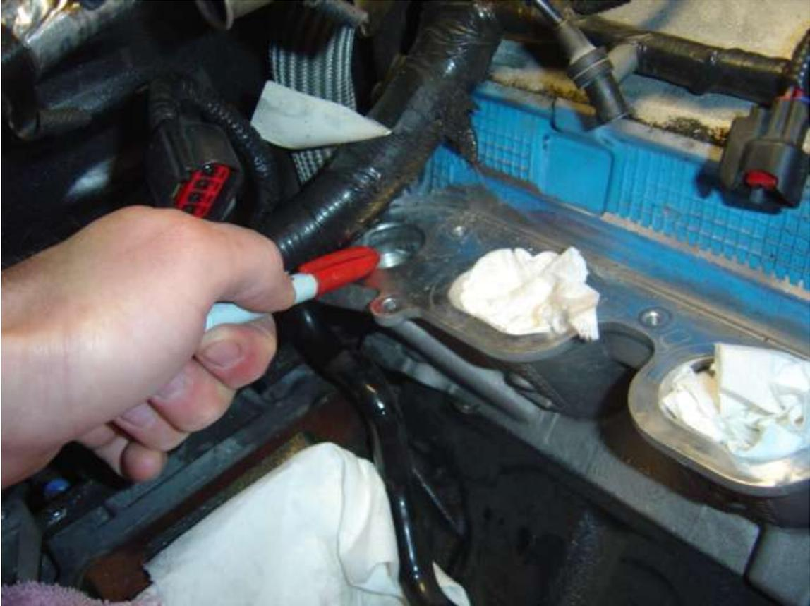
This fitting allows hot coolant to circulate from the driver's side rear head directly to the upper radiator hose for circulation through the radiator once the thermostat has opened. This coolant jacket is located directly behind the last intake manifold runner on the driver's side and has a freeze out plug installed from the factory.
