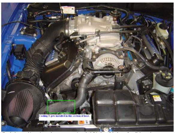
Cut the hose at this section and remove approximately 1.5 inches of the hose. Install the coolant "T" with the supplied clamps. The  $\frac{1}{2}$ " barbed fitting on the coolant "T" should point towards the valve cover. Leave clamps loose until final tightening.
