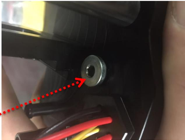
9. If you are only running two fuel pumps you will need to install the provided 4 ORB plug as pictured in the location where the third pump would reside.
