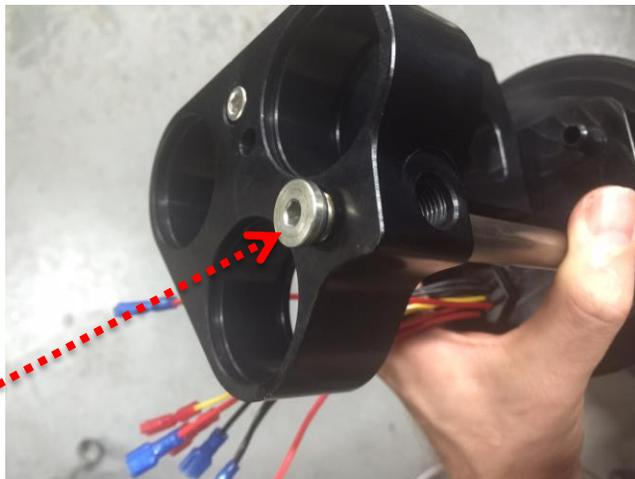
10. You also need to determine if you are planning a bottom exit or side exit fuel return location. We recommend the side exit as it seems to help with fuel aeration and tuning. In the picture the plug is installed on bottom so that the fuel will exit out the side. This is also a 4 ORB plug.
