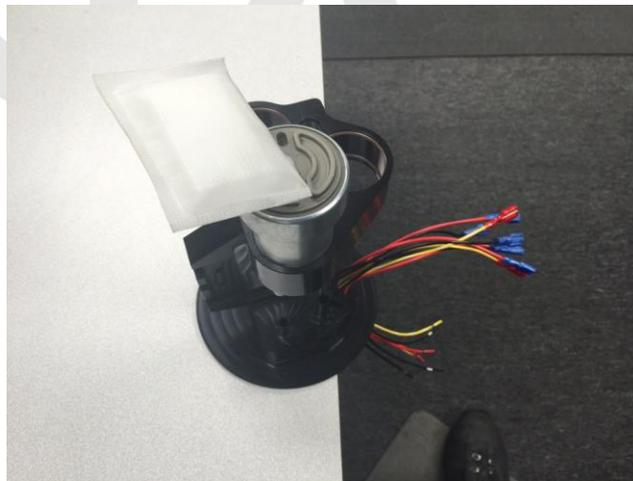
8. Install the fuel pump filter socks and insert fuel pump into the fuel hat. Verify the socks are  $\frac{1}{2}$ " to  $\frac{3}{4}$ " above the bottom of the tank and trim the hose as necessary. This can be done with a tape measure.
