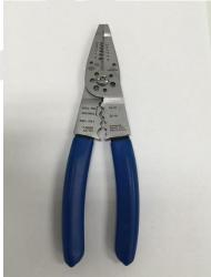
2. Using a set of wire strippers like the above will allow you to provide a secure crimp for the connectors and enjoy long term trouble free operation. These are available at hardware stores for \$15-25 if you don't already have a set.
