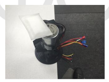
8. Install the fuel pump filter socks and insert fuel pump into the fuel hat. Verify the socks are ½" to ¾" above the bottom of the tank and trim the hose as necessary. This can be done with a tape measure.
