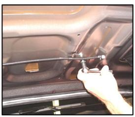
6. Install the four (4) flush plugs (PN: 9750K25) into the 7/8" holes drilled on the underside of the hood.
