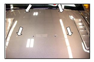
5. With a commercially available drill bit set (or a step drill bit), begin drilling the pilot holes open, working up to a size 7/16 IN drill bit. **Do not drill the second layer sheet metal pilot holes** open at this time.
