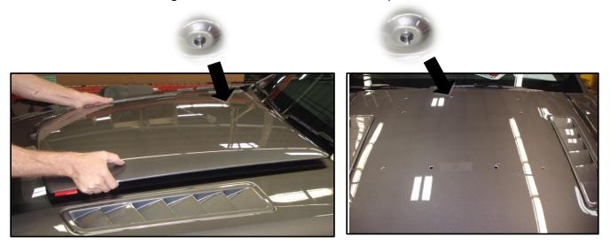
Center the hood scoop between the cowl lines of the hood. If the vehicle is equipped with heat extractors, center the hood scoop between the heat extractors.
