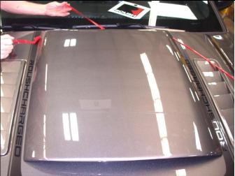
4. To properly set the tape, press firmly around the perimeter of the hood scoop.
