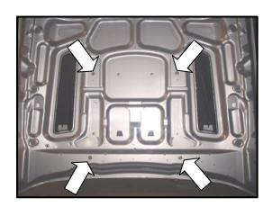
7. With commercially available clear coat, paint the exposed metal to prevent corrosion. (Motorcraft Part Number: PM-19500-6000)
