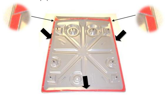
7. Pull approximately one inch of red tape from left, right and rear pieces of tape to allow for removal of tape once installed. Bend the tabs over for access to remove once hood scoop is in place.
