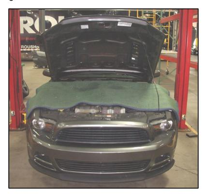
(Blanket will catch pins if dropped and metal debris while drilling.)
