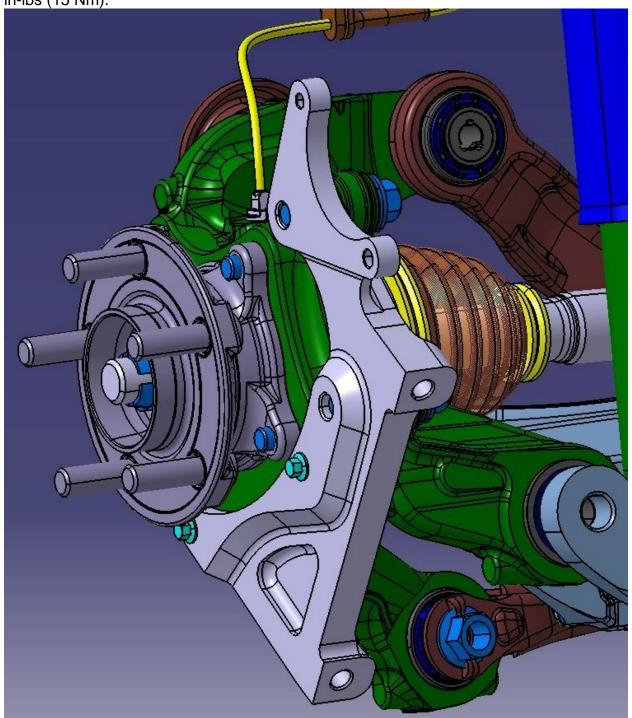
The hand-brake caliper is mounted using the M8 and M10 bolts included with the system. Torque the M8 bolt to 25 ft-lbs (34 Nm) and the M10 bolt to 35 ft-lbs (47 Nm). Connect the original cable to the new hand-brake caliper. Pull the hand-brake lever several times in order to bring the pads into contact with the disc.
