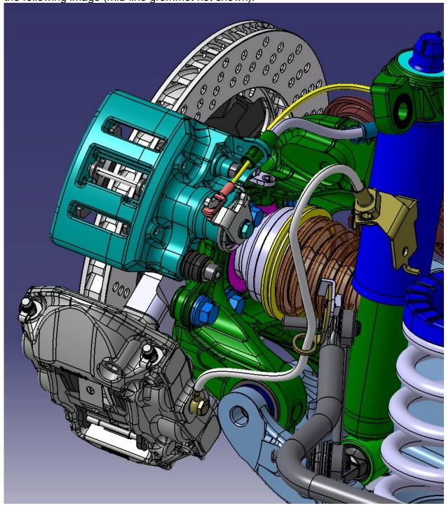
Due to the low mounting position of the main caliper, special care is needed in order to ensure that all of the air is purged from the system when bleeding. The caliper should be placed in a relatively vertical position when bleeding, while keeping a spacer between the pads to prevent the pistons from extending. When bleeding is complete, mount the caliper using the aforementioned torque specs.
