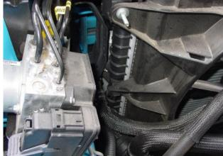
6 Remove the grommet from the stock air inlet removed in step 4 and insert it into the hole in the JLT heat shield. Slide heat shield on to the stud on the fan shroud and bolt down using stock air box bolt
