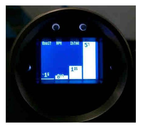
This graph mode displays the first 4 parameters programmed into cyclic scan or the 2 parameters from normal scan mode and the third and fourth from cyclic mode depending on how long the two buttons were held as described above. In most cases, the range of values (max height of each bar) will "grow" or adjust based on the max value observed. Some however are pre-set with a max range that should never be exceeded.
