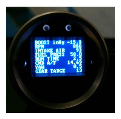
This screen will display the 8 parameters chosen in **Cyclic Scan**, or the two parameters that were last displayed in normal **Scan** mode plus the last 6 in **Cyclic Scan**.
