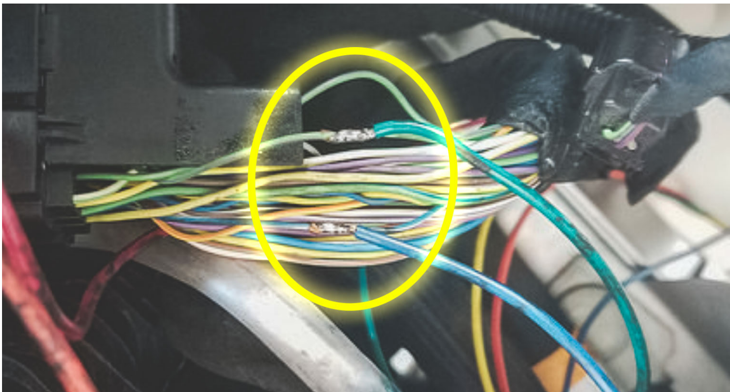
WOT Box BLUE and GREEN wires connected.
