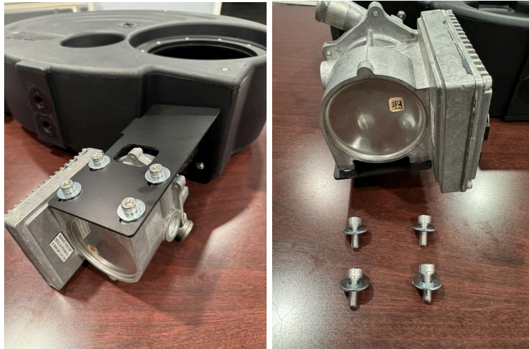
Figure 5: EMP bracket installation
