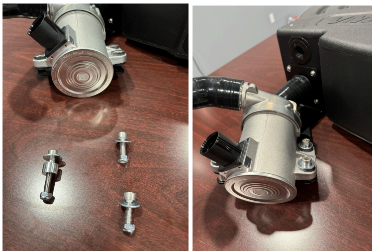
Figure 4: C-Max bracket installation
