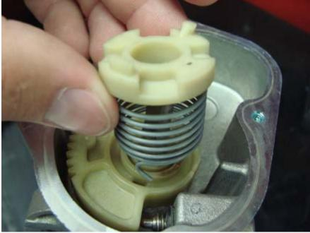
Install spring and plastic adapter to throttle body. \*\*Note that the tail of the spring locates into the hole in the brass gear.
