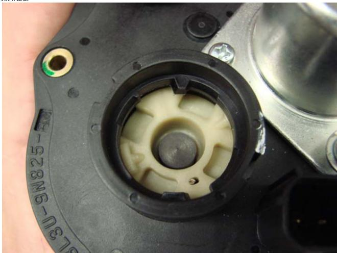
Using an Anerobic silicone such as Loctite #518, apply approx. 3mm bead around the throttle body mounting surface. Install throttle body to supercharger inlet housing using the factory (4) mounting bolts. If you are installing this throttle body on the Whipple 2.9L you will need to use shorter bolts than the factory ones. I believe Whipple provides them in the 2.9L kit.
