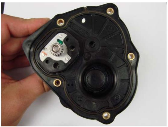
Install electric motor cover to new mono blade throttle body. Utilize the (5) factory torx bolts to secure in place. Install blue Loctite #242 to threads.
