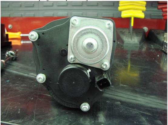
Using a small flat head screw driver, carefully remove the inspection cover from electric motor cover.
