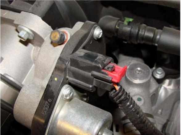
Remove throttle body from supercharger inlet housing by removing the (4) bolts that secure TB to SC inlet.
