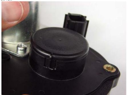
Remove the throttle spring and plastic adapter from throttle body. If this comes apart while removing cover from stock throttle body, then see picture below. The small end of the spring goes onto the plastic adapter. The spring locks into the plastic adapter with the tail of the spring locating into plastic adapter hole.
