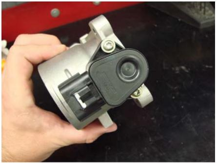
Remove TPS sensor from stock throttle body, install TPS sensor to new mono blade throttle body. Utilize the supplied (2) 4mm x 10mm allen bolts. Install blue Loctite #242 to threads.
