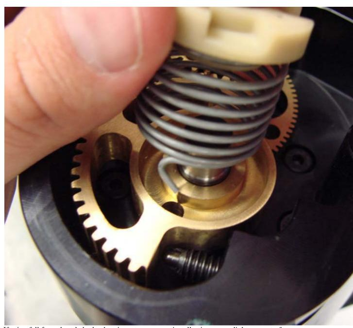
If oring fell from throttle body electric motor cover, reinstall using a very light amount of grease.
