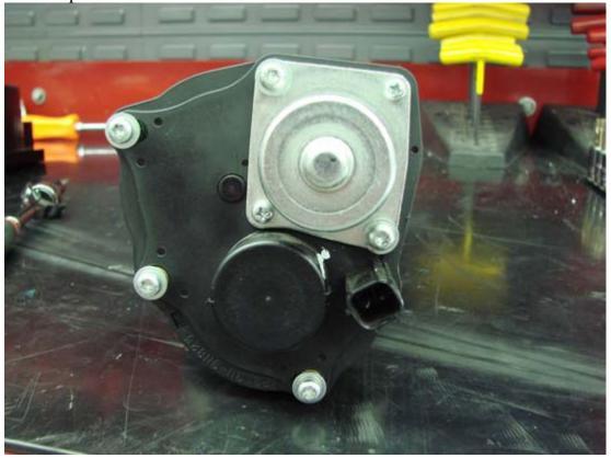
I did not use the spring rotation tool, because I bought the T/B used so I did not have it. However, I used a tiny screwdriver to push down on the tab and rotate it counter clockwise until it clicked into the tabs. The throttle body should spring back easily not snap back. Once it's into place you should also be able to push the throttle blade back just a little and have it spring forward.
