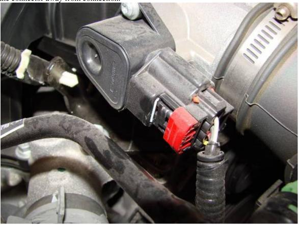
Throttle Position Sensor. Carefully pull red tab out, squeeze the connector and then pull the
