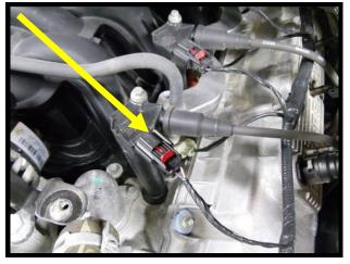
31. Disconnect spark plug wire from ignition coils (8) by pulling from ignition coil.
