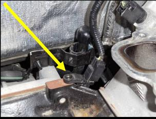
47. Remove heater hose tube from block by removing the (1) mounting bolt using an 8mm socket and pliers to remove clamp. There may be coolant left in this line, drain into clean bucket. This steel tube will not be reused. Remove tube from hose by using pliers to remove clamp.
