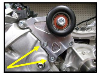
57. Install the supplied (1) 8mm x 50mm SHCS to the adjustable idler plate and water pump on passenger side.
