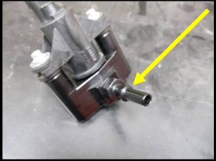
126. Install the BEVIS to the billet relocation bracket using the factory fasteners (8mm socket). Torque to 106 in/lbs.
