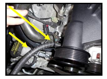
99. Reinstall the original factory ground wire to the alternator ground stud (13mm wrench). Press plastic cover back into place.
