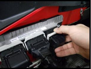
4. Remove plastic/rubber sealing gasket from factory PCM flange. This will be reinstalled when the PCM is reinstalled after the reflash.
