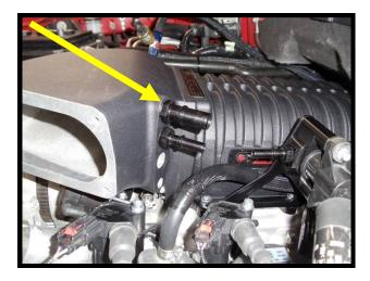
148. Install the -6AN to 3/8" barb aluminum quick connect fitting to the driver side of SC inlet, third hole from top.
