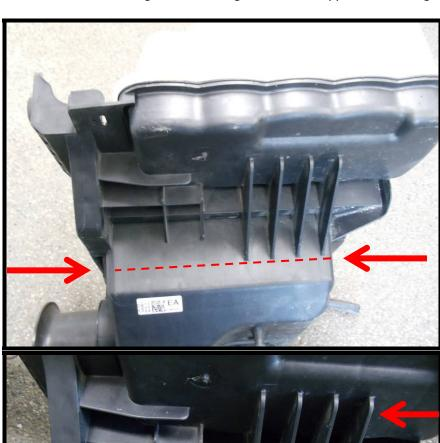
161. Cut/grind the front side of the coolant reservoir you previously cut, to a smooth flat surface as shown in the image.
