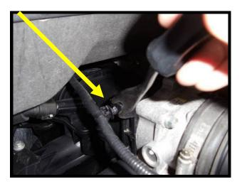
18. Disconnect the BEVIS electrical connector by pressing in the tab and pulling (tab on backside of connector). Then remove the quick connect fitting from BEVIS barb fitting. To unlock tab, release lock and pull towards firewall.
