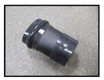
173. Install air inlet tube to connect air box to the MAF. Slide rubber hoses into place. Secure with supplied #80 hose clamp (5/16" nut driver).
