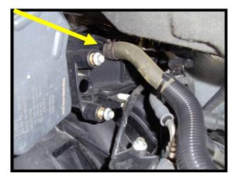
21. Pry the white plastic connector holding BEVIS electrical wires to intake manifold.
