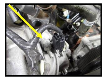
54. Remove white plastic clip from capacitor. Rotate capacitor and reinstall plastic clip as shown in image. This is for clearance when mounted to the idler plate.
