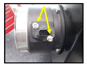
169. Install MAF body to new air box as shown in image, use the (4) 6mm x 16mm SHCS and the billet venturi from the inside of the air box (5mm allen). Torque to 95 in/lbs.
