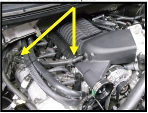
151. Install the supplied 3/8" ID x 15" rubber hose (with dual 90deg quick connect fittings) between the BEVIS and the 3/8" barb fitting on the SC inlet. Route underneath coil wires, push fitting over aluminum fitting until it clicks and locks into place.
