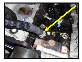
84. Secure both heater hoses using zip-ties for a nice clean installation.
