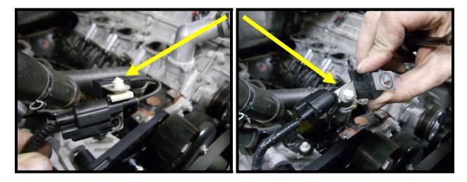
55. Install the supplied adjustable idler pulley bracket to the passenger side of engine as shown in image. Use the ([1 of 3] 8mm x 60mm SHCS) and the (1) 8mm AN washer to the capacitor hole and idler plate. Install capacitor to the backside of bolt and washer so that it's mounted against idler plate. Torque to 22 ft/lbs.
