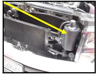
78. Install the supplied 7/32'' ID x 27.5'' rubber hose to the intercooler reservoir nipple. Route down behind heat exchanger bracket on driver side, down to the frame rail. There's a small hole by the chassis mount. Route through this hole as shown in image. This is only a vent.
