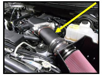
174. Install the 5/8" aluminum barb fitting into the rubber grommet installed in air inlet tube.
