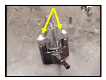
127. Install the BEVIS relocation assembly to the steel bracket using the supplied (2) 6mm x 18mm SHCS (5mm allen). Torque to 106 in/lbs.
