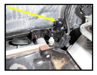
46. Remove the factory bolt (1) that secures the crank position sensor (8mm socket). Install the supplied (1) 6mm x 20mm low head socket cap using a 5mm allen wrench. Torque to 106 in/lbs.
