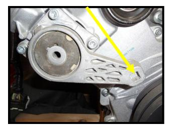
24. Disconnect the 3-way electrical connector from alternator. To unlock, squeeze connector and pull up.
