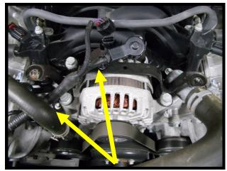
27. Carefully cut the electric tape holding the alternator wiring to the radiator shroud (plastic clip). Remove clip from radiator shroud.
