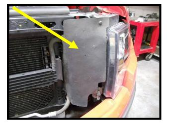
60. Remove (2) plastic push pins from passenger side rubber shielding from headlight/front clip as shown in image. The passenger side heat exchanger bracket will slide behind this.
