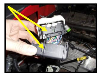
107. Install supplied split loom over the 2-way charge air temp sensor pigtail for protection. Install electric tape on both ends so loom can't come off the ends.
