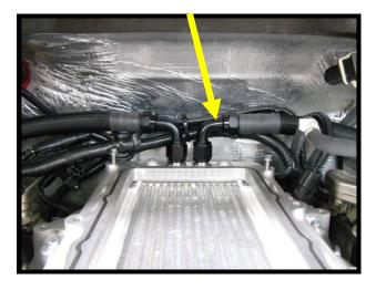
116. Route 5/8" ID x 54" IC return line along firewall to the IC reservoir 5/8" return nipple. Secure to IC reservoir with (1) #16 pinch clamp.
