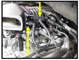
152. Remove rubber ½" ID hose from brake booster line and check valve assembly as shown.
