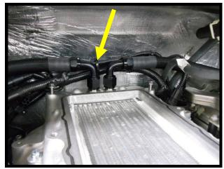
124. Reconnect the factory fuel feed line to the factory fuel rail by pressing until it clicks and locks.
