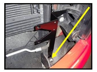
68. Carefully tighten the headlight/front clip bolt that secures the top of heat exchanger bracket on driver side (10mm socket). Be cautious of stripping the threads.
