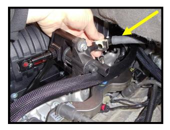
142. Connect the BEVIS 2-way electrical connector to BEVIS, push until it clicks and locks into place.
