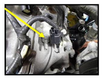
53. Remove the (1) capacitor bolt on the passenger side using a deep-well 18mm socket.
