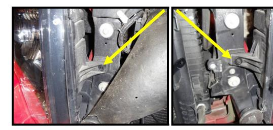
63. Route the passenger side heat exchanger bracket through the rubber shielding. Secure bracket with factory headlight/front clip bolt. Leave slightly loose for now.
