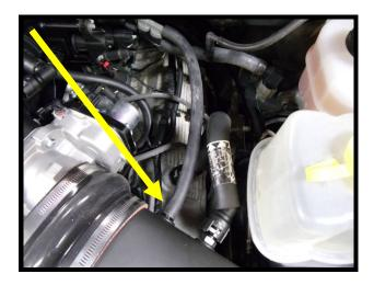
178. Install the coolant reservoir vent line down the fender, to the factory radiator fill cap.
