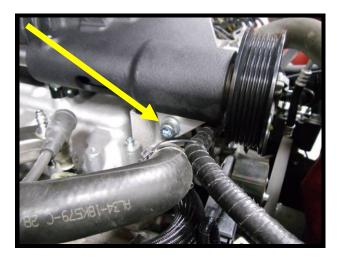
138. Reinstall the factory ignition coils using the (8) 6mm x 90mm SHCS (5mm allen), (8) 8mm AN washers and the supplied 1.75" billet spacers. Note: There are 4 driver side coils, 4 passenger side coils, do not mix up. Torque to 106 in/lbs.
