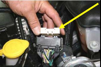
103. Remove the PCM connector strain relief from backside of connector so you have full access to the wires.
