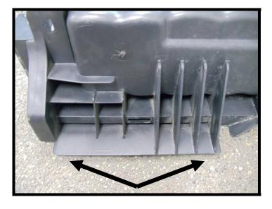
163. Install the supplied cold air box mounting spuds to the bottom of the air box. Use the supplied (2) 6mm x 22mm SHCS through the spud. Secure spud on filter side with the supplied (2) 6mm Nyloc nuts and (2) 6mm AN washer.
