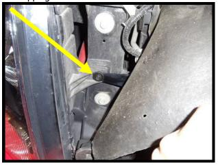
66. Install the driver side heat exchanger bracket to frame rail and headlight/front clip. Secure top with factory bolt but leave loose until bottom mount is started.
