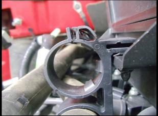
13. Remove the rubber hose from the brake booster check valve assembly to the air intake plenum.
