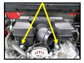
12. Release the factory rubber heater lines from factory plastic clamp on air intake plenum. To release the clamp, use a small pick through the side of it, press tab down and it will release.
