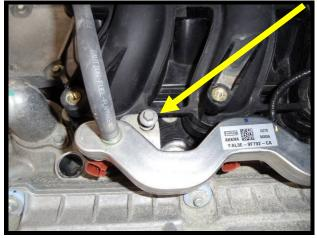
36. Remove the safety clips securing the fuel injectors to fuel rail by pulling away from open end. Remove fuel injectors from factory fuel rail, these will not be reused.
