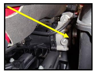
11. Using a 10mm socket, remove the bolts (2) securing the air intake plenum to the support bracket.
