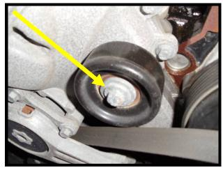
50. Remove the factory bolt that secures the water pump (1) to the block (10mm socket).
