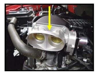
155. Route the throttle body 4-way connector under the throttle body and connect to throttle body TPS sensor. Connect by pressing together until it clicks and locks. Use a small zip-tie to secure throttle extension harness to factory harness.
