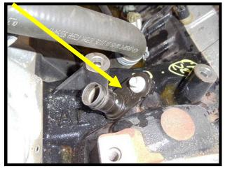
49. Remove factory 76mm idler pulley from passenger side of engine (above spring loaded tensioner) using a 13mm socket.
