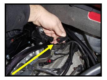
143. Connect the bypass valve's vacuum/boost actuator rubber hose by connecting the ¼" barb from the bypass actuator to the ¼" barb installed in runner just below it. Use the supplied (1) ¼" ID x 3" to connect the two barbs.
