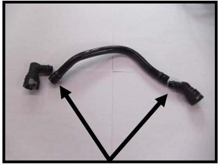
150. Install the 90deg and 45deg quick connect fittings from PCV tube to the new supplied 5/8" ID x 14" rubber hose. Connect the 90deg fitting back to passenger side valve cover, and connect 45deg fitting to Whipple fitting on passenger side of inlet. Push until it clicks and locks into place.
