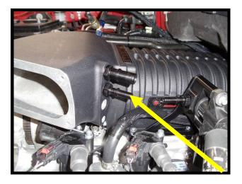
149. Use a razor blade to cut the factory shielding from the PCV line. Once removed, use a razor blade to carefully cut the factory quick connect fittings (1-90deg and 1-45deg) from the factory PCV tube. Note: There is an oring towards the bottom of the barb fitting, do not go through it. You can cut through the top area and then pry fitting out without ever touching the oring.
