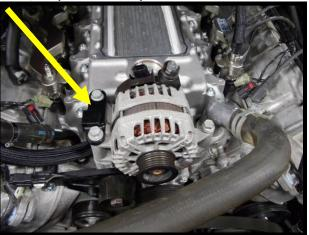
98. Pre-route the alternator ground wire and alternator 3-way connector along the heater line (this is for pulley/belt clearance). Use zip-tie to secure wires to heater lines for extra belt/pulley clearance. Note: Image shows with SC assembly installed to show best possible position.
