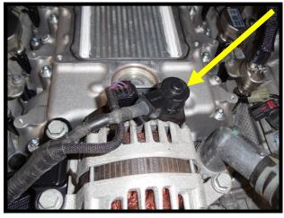
100. Reconnect alternator 3-way connector to alternator until it clicks and locks into place.
