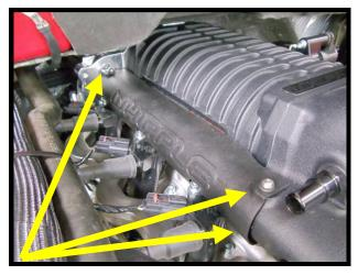
145. Install the supplied 3/8" ID x 51" fuel line hose with protective mesh covering to the factory cross-over barbs. Install on driver side first, by pressing onto barb and securing with supplied clamp (1 of 2) (7mm socket). Route behind the BEVIS relocation assembly and around the back of the SC (against firewall). Route along engine on passenger side and secure to passenger side fuel rail barb. Secure hose with supplied clamp (1 of 2) (7mm socket)
