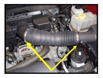
7. Remove the factory MAF sensor element from the factory air box lid. Utilize a T20 torx socket or wrench to remove. This will be installed later into the new MAF housing.
