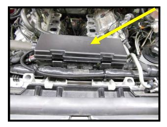
113. Run main power wire from intercooler relay harness along radiator shroud (secure with zip-ties for clean installation) to the main fuse box. Come through the passenger side opening. Remove the factory nut from the power stud in the box. Install the power eyelet from the IC relay harness to this stud. Reinstall factory nut to the power stud until tight.
