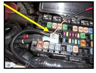
114. Pull the yellow 20amp fuse from position #78. Install the 20amp yellow fuse in the unused fuse slot on the fuse tap. Install the supplied fuse tap into position #78. Note: 20amp yellow fuse should be in bottom slot, 5amp should be in top slot.
