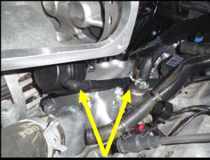
144. Install the supplied jack-shaft cover to passenger side of supercharger. Use the supplied (3) rubber grommets (insert into plastic cover 3 holes (1 is left empty) and (3) 5mm x 12mm BHCS. (2) go to the front holes, (1) goes to the back top hole.
