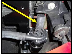
77. Install the supplied intercooler reservoir to driver side heat exchanger bracket using the supplied (2) 8mm x 25mm flanged hex head bolt. Slide reservoir bottom nipple into 3/4" ID hose from IC pump, secure with pinch clamp. Torque to 22 ft/lbs.
