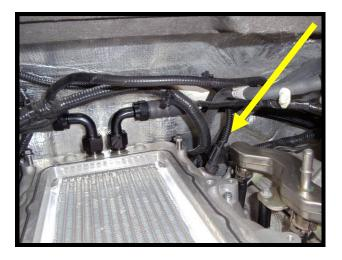
120. Install the throttle body 6-way extension harness to factory 6-way connector by pressing together until it clicks and locks. Lock the red safety lock by pressing until it clicks and locks.
