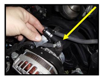
26. Pry plastic clips (3) from air intake plenum support bracket and alternator ground wire. Remove the alternator ground wire by removing the (1) nut (13mm socket). Cut these clips from the wiring harness, they will not be used.
