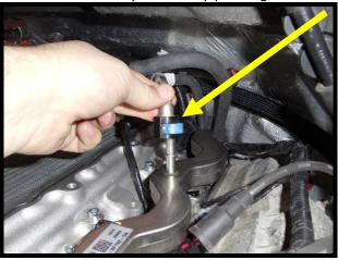
125. Install the supplied –6AN viton orings (4 of 4) to all the –6AN to 3/8" barb fittings. Install (1) of the –6AN fitting to 3/8" barb black fitting into BEVIS billet bracket.
