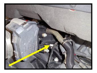
22. Pry plastic clips (4) from intake manifold on backside of engine, (2) passenger side and (2) driver side.
