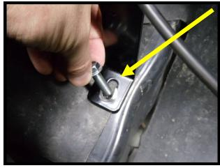
65. Carefully tighten the headlight/front clip bolt that secures the top of heat exchanger bracket on passenger side (10mm socket). Be cautious of stripping the threads.
