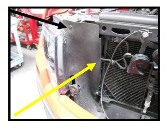
61. (MY2010) Use the supplied 8mm x 1.25 tap to tap the factory frame rails for the heat exchanger mounting brackets. Apply light amount of cutting oil or engine oil to prevent galling.
