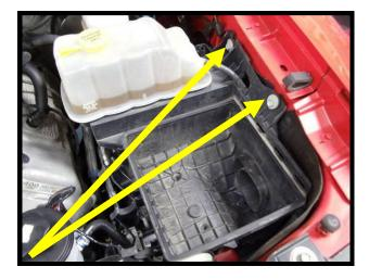
44. Remove factory air filter rubber shielding by prying out the (6) plastic push pins.
