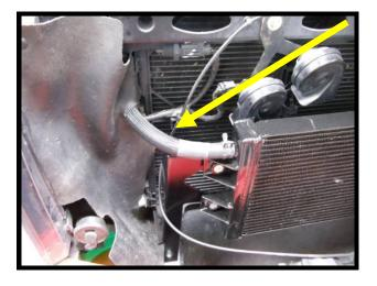
119. Pre-route the inlet air temp sensor 2-way connector to the driver side and connect to air temp sensor. This must go along the firewall to clear SC assembly.
