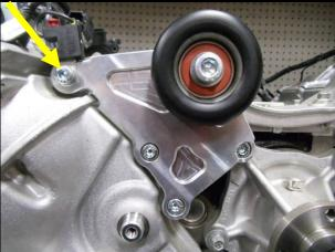
56. Install the supplied ([2 of 3] 8mm x 60mm SHCS) to the adjustable idler plate and timing chain cover on passenger side. Torque to 22 ft/lbs.
