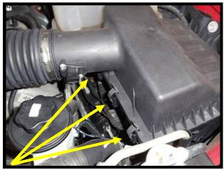
9. Disconnect the quick disconnect vent line from the passenger side of the air intake plenum. Disconnect vent line from valve cover as well. To release quick connect fittings, press tab clock-wise which will release fitting. The fittings will be used at a later step.
