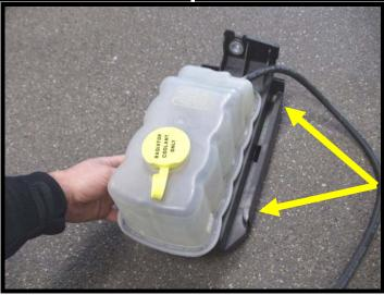
162. Cut/grind the back side of the coolant reservoir you previously cut, to a smooth flat surface as shown in the image.
