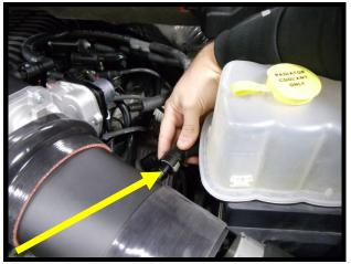
176. Install the 3/8" plastic barb fitting into the 3/8" ID rubber hose from the brake booster.
