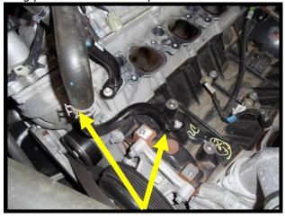
48. Install the supplied short steel heater hose tube to the factory location using the factory bolt (8mm socket). Torque to 106 in/lbs.
