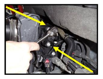
20. Remove the rubber brake booster hose from intake manifold by releasing hose clamp and pulling hose.
