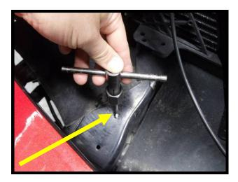
62. Remove the (2) bolts securing the headlights to the front clip as shown in image (10mm socket).
