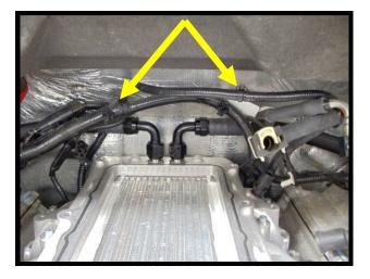
123. After pre-routing electrical wires towards the firewall, use zip-ties to secure wires together and then tuck behind the IC fittings/hose. This will allow the SC to slide into place easier. Make sure to pull wires towards driver side to give enough slack later.
