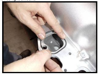
90. Install intake manifold assembly to engine by carefully setting into position. Ensure that the bolts holes line up and the manifold can move freely.
