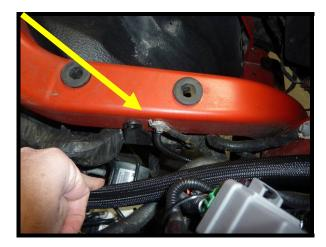
112. Open the factory fuse box lid on top, center of the radiator shroud.
