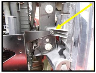
67. Install the supplied 8mm x 25mm flanged hex bolt (1 of 2) into driver side of frame rail to secure bottom of heat exchanger bracket. Sandwich the rubber shielding under the bracket to secure it. Carefully tighten bolt, be cautious of stripping the threads.
