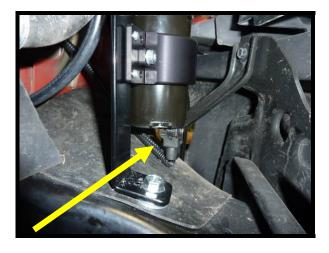
111. Remove the factory ground bolt from the frame rail (inner-side), very near the rubber air filter box grommets. Install the intercooler relay harness ground wire/eyelet to this bolt and factory eyelet. Reinstall the factory bolt and secure to frame rail until tight.
