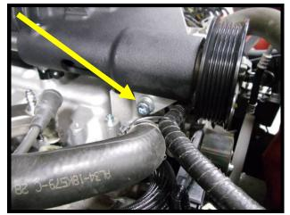
134. Install the BEVIS relocation assembly to the supercharger assembly using the supplied (2) 8mm x 25mm SHCS (hand tight).
