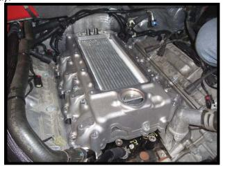
91. Reinstall the factory alternator mounting bracket to the block using the factory flanged hex head fasteners (4) 8mm x 54mm (10mm socket). To install back passenger side bolt, slightly lift intake manifold and drop bolt in place. Torque to 22 ft/lbs.
