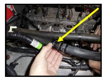
83. Route ¾" ID rubber heater hose down along the line of other factory heater hose, install end onto previously installed ¾" ID barb in the valley of the block. Secure with supplied #16 pinch clamp.
