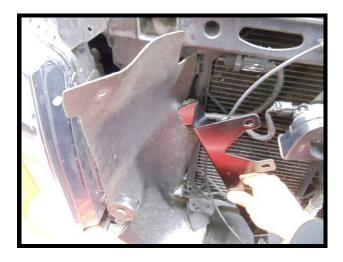
64. Install the supplied 8mm x 25mm flanged hex bolt (1 of 2) into passenger side of frame rail to secure bottom of heat exchanger bracket. Sandwich the rubber shielding under the bracket to secure it. Carefully tighten bolt, be cautious of stripping the threads.
