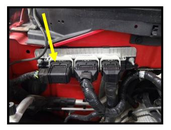
102. Remove the pin-locking device from the connector using a small screw driver or pick.
