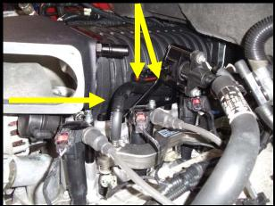
146. Install the -6AN to 5/8" barb (1 of 2) aluminum quick connect fittings to the passenger side of SC inlet.
