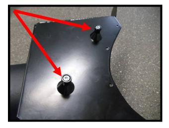
165. Install cut coolant reservoir to the new air box for mockup. Install factory bolt in the top support/fender. Hold the reservoir up against the air box and mark the (3) holes from the air box to the coolant reservoir. The measurements should be roughly 1 ¼" down from ledge, and the (3) holes should roughly be 1 ¾", 3 ¾", 6 ¾" from the ledge (fender side) as shown. Remove coolant reservoir and use a 1/4" drill bit to drill these (3) holes.
