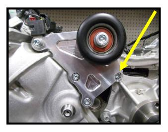
58. Reinstall the factory 76mm steel idler pulley to the factory location (13mm socket). Torque to 22 ft/lbs.
