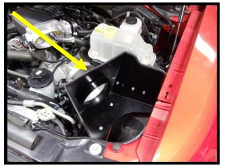
171. Install supplied air filter to the venturi ring using the supplied #104 hose clamp (5/16" nut driver). Position hose clamp so the nut area is hidden on the backside.
