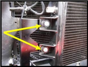
73. Install intercooler electric pump clamp to driver side heat exchanger bracket by mounting from the back side (2) 6mm x 12mm flanged hex head bolts. Torque to 106 in/lbs.
