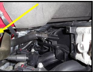
10. Loosen the hose clamp connecting the air intake plenum to throttle body using a flat head screw driver or 5/16" socket.
