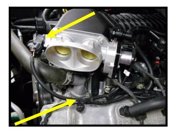
156. Connect the throttle body electronic control 2-way connector (extension) to electronic throttle motor. Push together until it clicks and locks into place.
