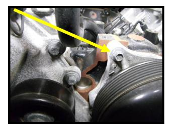
51. Remove the (2) bolts that secure the timing chain cover, passenger side (2) to block (10mm socket).
