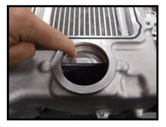
131. Pre-install (2) of the 8mm x 20mm 6-point bolts in the back 2 bolt holes. Insert these 6-point bolts 1 rotation as the SC assembly will be slid into position using these to locate it.
