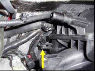
23. Using a ½" breaker bar, release tension from factory tensioner by rotating the breaker bar in a clock-wise rotation. Remove factory serpentine belt from engine once belt has extra slack.
