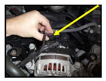
25. Open the plastic connector on the alternator ground wire. Using a 13mm socket, remove ground wire from alternator stud.
