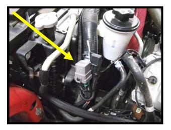
110. Run the 2-way connector and loom through the radiator support and plug connector to pump. Push connector on until it clicks and locks into place.
