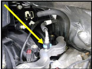
35. Remove the (4) mounting bolts holding the factory fuel rail on (8mm socket). Pull fuel rail from intake manifold.
