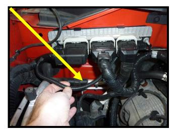
109. Mount the intercooler relay and fuse harness to the factory plastic loom coming down the radiator from main fuse box, driver side. Use a zip-tie to secure to loom.
