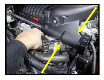
137. Torque the (1) 10mm x 30mm SHCS in the SC front support to 25 ft/lbs.
