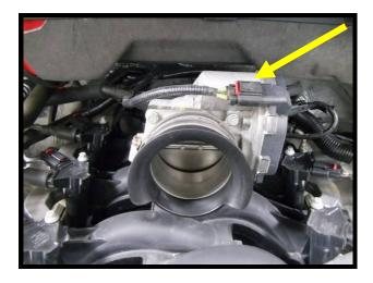
17. Pry the plastic connector holding the electronic throttle body wires to the intake manifold from manifold.
