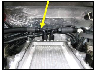
118. Route 5/8" ID x 62" IC feed line through the rubber shielding between passenger side headlight and radiator, to the heat exchanger 5/8" nipple. Secure hose with supplied (1) #16 pinch clamp.
