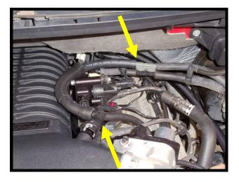
154. Install supplied throttle body to supercharger inlet along with the supplied throttle body gasket. Use the (4) 6mm x 25mm and (4) 6mm AN washers to secure throttle body to SC. Torque to 106 in/lbs.
