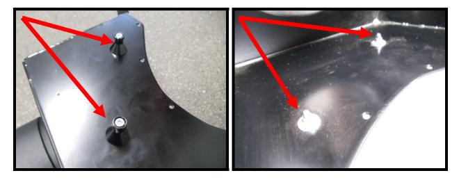
164. Mount air box to factory location by dropping aluminum spuds into factory rubber grommets. Apply light amount of oil or silicone to help the spuds slide in.
