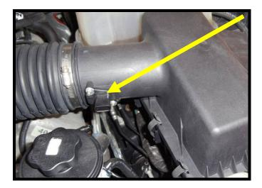
8. Loosen the factory air box lid by pushing the (3) locking tabs back. Lift air box lid from air box, this will not be reused.
