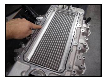
130. Apply light amount of grease on the manifold bypass oring, located in the 2.5" bypass hole. This is to help prevent ripping the oring during the installation process.
