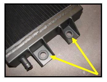
70. Install the supplied (4) aluminum heat exchanger spuds to rubber grommets installed in heat exchanger.
