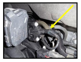
19. Remove BEVIS from engine by removing the (2) bolts (8mm socket). Disconnect quick connect fitting from BEVIS by squeezing white tabs on bottom of connector. The BEVIS will be reinstalled later in manual.
