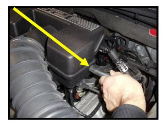
14. Disconnect the quick connect vent line from the driver side plenum. To release, press tab down and pull.
