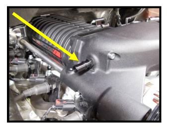
147. Install the -6AN to 5/8" barb (1 of 2) aluminum quick connect fittings to the driver side of SC inlet, top hole.
