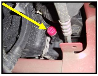
3. Remove the PCM from the passenger side of firewall by disconnecting the 3 main connectors (pull back on gray tabs) and removing the 2 mounting bolts (10mm deep-well socket).
