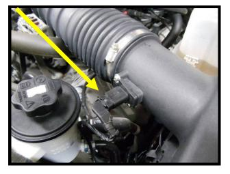
6. Loosen hose clamps (2) that are securing the air inlet tube to the factory air box and intake plenum. Utilize a 5/16" nut driver. Remove air inlet tube, this will not be reused.
