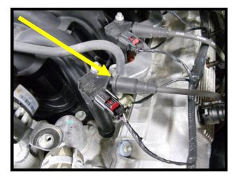
32. Remove ignition coils from engine by removing the each mounting bolt (1 per coil), utilize an 8mm socket to remove bolt.
