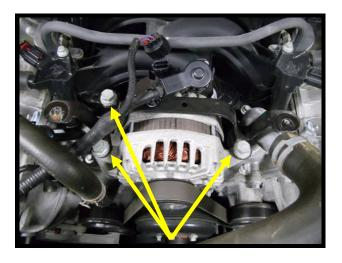
29. Remove alternator mounting bracket by removing the (4) mounting bolts (10mm socket).
