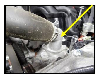
43. Remove air box and coolant reservoir from fender by removing the (2) mounting bolts (13mm socket) and removing rubber vent line from radiator fill cap barb.
