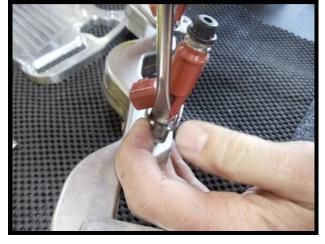
37. Using a razor blade, carefully cut the factory fuel crossover line at both barbs. Remove fuel line from fuel rail, this will not be used.
