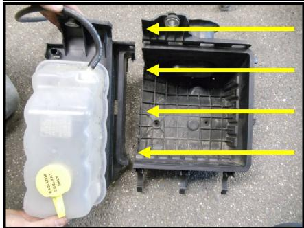
160. Mark the coolant reservoir back side straight across along the bottom supports. Cut straight across as shown in the image.
