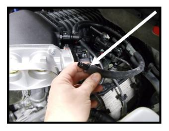
177. Install 3/8" rubber line from brake booster to air inlet tube and 3/8" plastic barb fitting.
