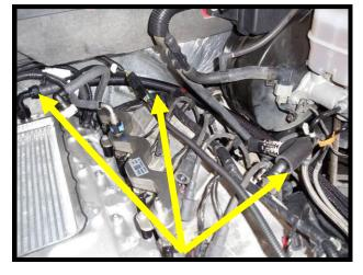
117. Install the supplied 5/8" ID x 62" rubber hose with the 90deg -10AN fitting (1" wrench) to passenger side intercooler fitting. Tighten -10AN fitting so the fitting is 90deg from the front of the vehicle (face towards passenger side).
