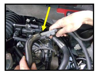
153. Install supplied 15/32" ID rubber hose by pressing hose end onto check valve assembly barb. Install 90deg fitting onto top 5/8" quick connect fitting installed on supercharger inlet.
