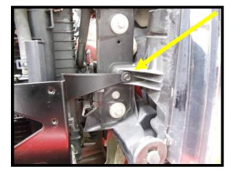
69. Install the supplied (4) rubber grommets to the heat exchanger mounts.
