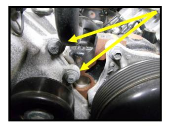
52. Remove the (1) nut from capacitor bolt on the passenger side using a 13mm wrench.
