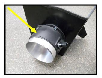
170. Mount the air box/coolant reservoir assembly back into factory location, locating on the (2) aluminum spuds into the rubber grommets.
