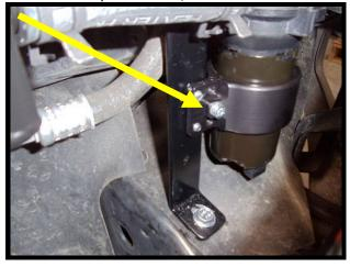
74. Install the supplied 34" ID x 4.25" rubber hose and supplied #16 pinch clamp to intercooler pump outlet.
