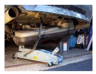
• Lower the tank a much as you can while making sure no lines are being stretched. Wiggle the tank around so its not resting on your exhaust or anything else while you lower it. (As you can see the jack has been moved and the wood is no longer there)
