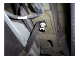
• Remove the three 13mm bolts holding up the tank. When you remove the bolts the tank still might not lower, this is because of the sticky puddy on top of the tank toward the rear. I took a screw driver and a sliced through the puddy which allowed the tank to drop.
