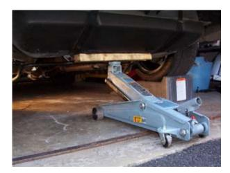
• Support the tank with a jack, the wood isnt really necessary and I ended up moving the lift around as I lowered the tank. The tank was also a little less then 1/4 full, so I was able to hold it up with one arm and move the jack around.
