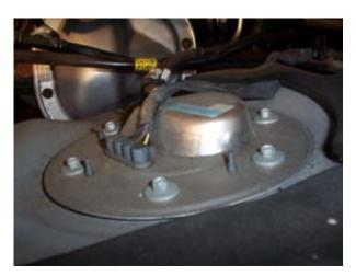
• Remove the six 8mm bolts holding the tank cover on.
