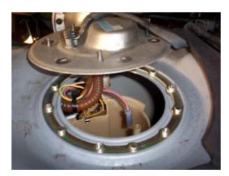
• Take the wire harness out of the stock pump by pushing in the tab (use a flat head screw driver) thats facing toward the front pass side of the car. If you cant find it then look on the Focus pump assembly and youll see it. CAREFULLY remove the six 5mm screws holding the basket cover and hose on, then remove the cover by pushing the white tabs together and pulling off the cover. Now you can just pull the stock pump out.
