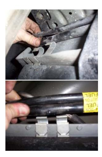
• Pull the hoses off of the little hooks. There are three places you need to do this, on the left and right side of the tank and in front of the tank facing the front of the car.
