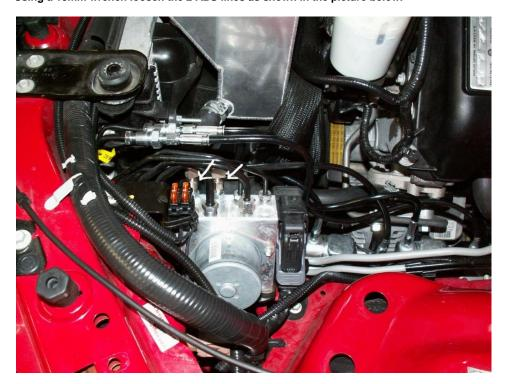
Once the those fittings are loose you can remove the fitting and hardline from the ABS block. Now you're going to install the (2)  $65307 - 3 \times 10$ mm x 1.0 IF Brake Adapter fittings into the ABS block using Teflon paste. Make sure to install them so that the -3an male flare is pointing up.
