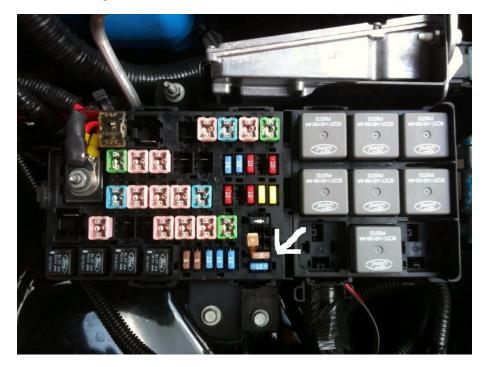
Take the stock fuse out, put in the atc fuse tap and reinstall the stock fuse in the fuse location on the fuse tap. Use the supplied 14ga wire and attach it to the atc fuse tap with the supplied female spade connector. Run that 14ga wire along the radiator shroud toward the drivers side of the car. You can use the supplied wire loom to cover the wire once it's been run for a cleaner look. Now attach the power wire to both blade fuse holder wires with the supplied 14ga butt connector.
