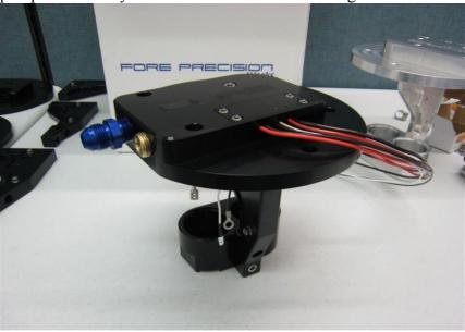
If you are installing the Dual FPDM Kit on an OEM Fuel Hat we suggest you try to modify it using a method similar to the one located in this thread. It's the most efficient and safest way to do so and avoid any fuel leaks.
