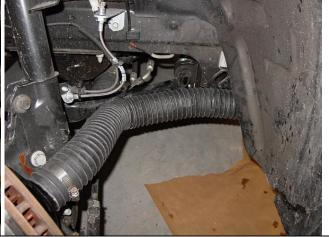
Repeat process for opposite side and check clearance between the hose and tire.
