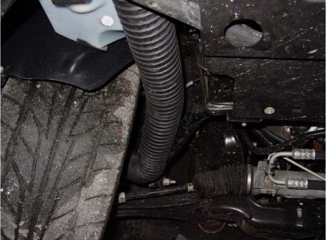
Reassemble brakes and wheels in reverse and you are done. Don't forget to re torque your lug nuts after a few miles of driving. We suggest 100 ft lbs.
