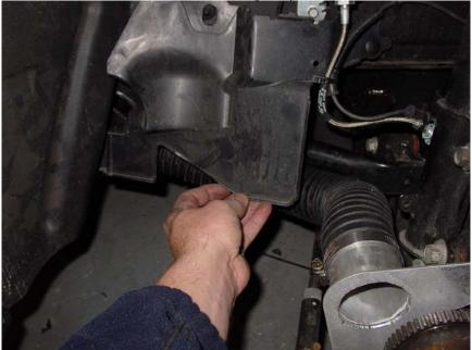
Using your drill and the 2 ¼" hole saw, drill from the back side of the bumper through the grille. Using a small angle drill or flexible extension will help. You can remove the bumper if you do not have the angle drill. You can also use a small air ratchet and socket if your hole saw has a hex shaft. See picture. If you purchased the JLT Bezels snap them in now.
