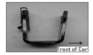
**Note:** Kit contains **2** different sizes of *U-Brackets*; two **narrow** and two **wide**. The **narrow** *U-Brackets* are to be installed in the **outermost** tabs of the fascia. The **wide** *U-Brackets* are to be installed in the **innermost** fascia tabs.
