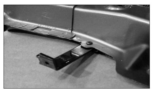
14. Install one *U-Nut/Clip* onto both *Short L Brackets*, on the side of the L Bracket that has the slotted hole. Face the threaded side of the clip towards the inside of the "L".
